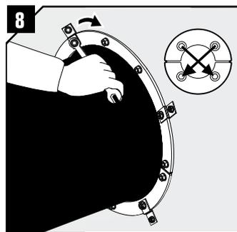
Tighten the bolts crosswise. The seal will compress and seal the transit. Please see table for recommended max torque.
