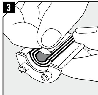
Adapt the seal to the cable/pipe by peeling off layers from the halves until you reach the gap seen in pic.4.
