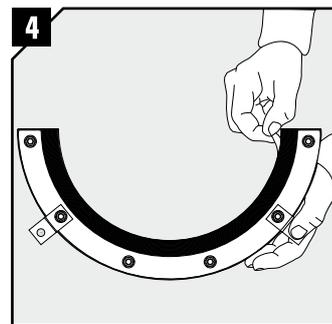
Adapt the seal to the cable/pipe by peeling off layers from the halves until you reach the gap seen in pic.5.
