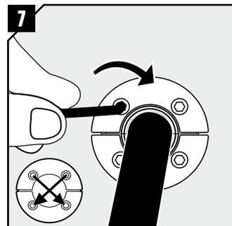
Tighten the screws crosswise. The seal will compress and seal the transit. Please see table for recommended max torque.
