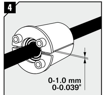
Try to achieve a 0-1.0 mm gap between the two halves when held against the cable/pipe.
