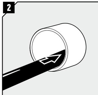
Pull the cable/pipe through. Please see note and table for aperture dimensions.
